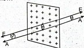
To calculate the electric intensity E at a point P, close to the sheet, imagine a closed Gaussian surface in the form of a cylinder passing through the sheet, whose one flat face contains point P. From symmetry, we can
