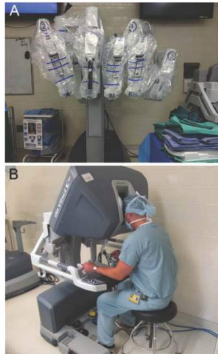
FIG 2 • A. The robot is draped sterilely. For a left-sided resection, arm 3 is placed as shown while arm 3 is moved to the opposite side for a right-sided resection. The surgeon operates with arms 1 and 2 while arm 3 is used for retraction. The joint of the camera arm ( arrowhead ) should be placed opposite of arm 3 to minimize bumping of the robotic arms. B. The surgeon sits at the console, whereas an experienced bedside assistant changes the robotic instruments, passes the staplers, and suctions when needed.
