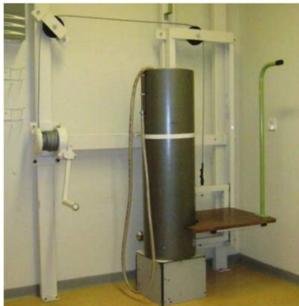
FIG 2 • Water reservoir for measuring the volume of a limb. On the right is the elevator to bring the patient up to the required height. The elevator handle is on the left.
